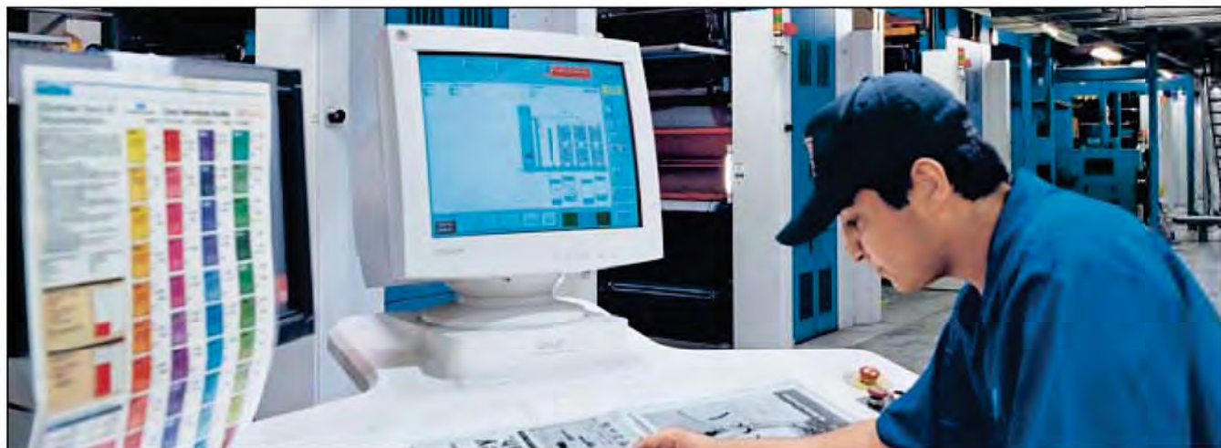
FIGURE 1. Windows operating systems are widely utilized in industrial automation, providing a familiar foundation for a human-machine interface (HMI)
