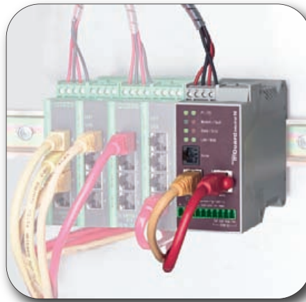
Figure 1. An mGuard Industrial RS for mounting on DIN rail with optional integrated analog modem or ISDN terminal adapter
